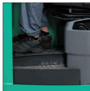
Adjustable floor plate
