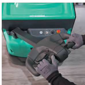
Easy-to-operate tiller arm
