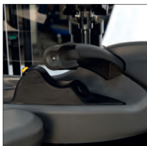
Ergonomic handle with drive control
